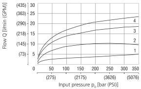
Nominal flow 8 l/min (2.1 GPM)
