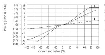
$Q_p = 8 \text{ l/min } (2.1 \text{GPM}) \text{ by } \Delta p = 10 \text{ bar } (145 \text{ PSI})$
