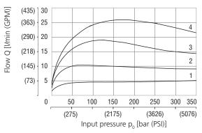
Nominal flow 15 l/min (4.0 GPM)
