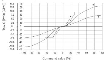
$\Delta \mathbf{p}$  = Valve pressure differential (inlet pressure  $\mathbf{p}_{v}$  minus load pressure and return pressure p<sub>¬</sub>)
