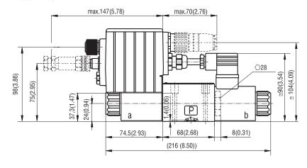
$PRM7\text{-}063 \dots E02501$  - without connector plug for spool position feedback  $PRM7\text{-}063 \dots E04501$
