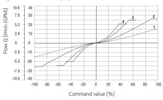
$Q_n = 30 \text{ l/min } (7.9 \text{ GPM}) \text{ by } \Delta p = 10 \text{ bar } (145 \text{ PSI})$
